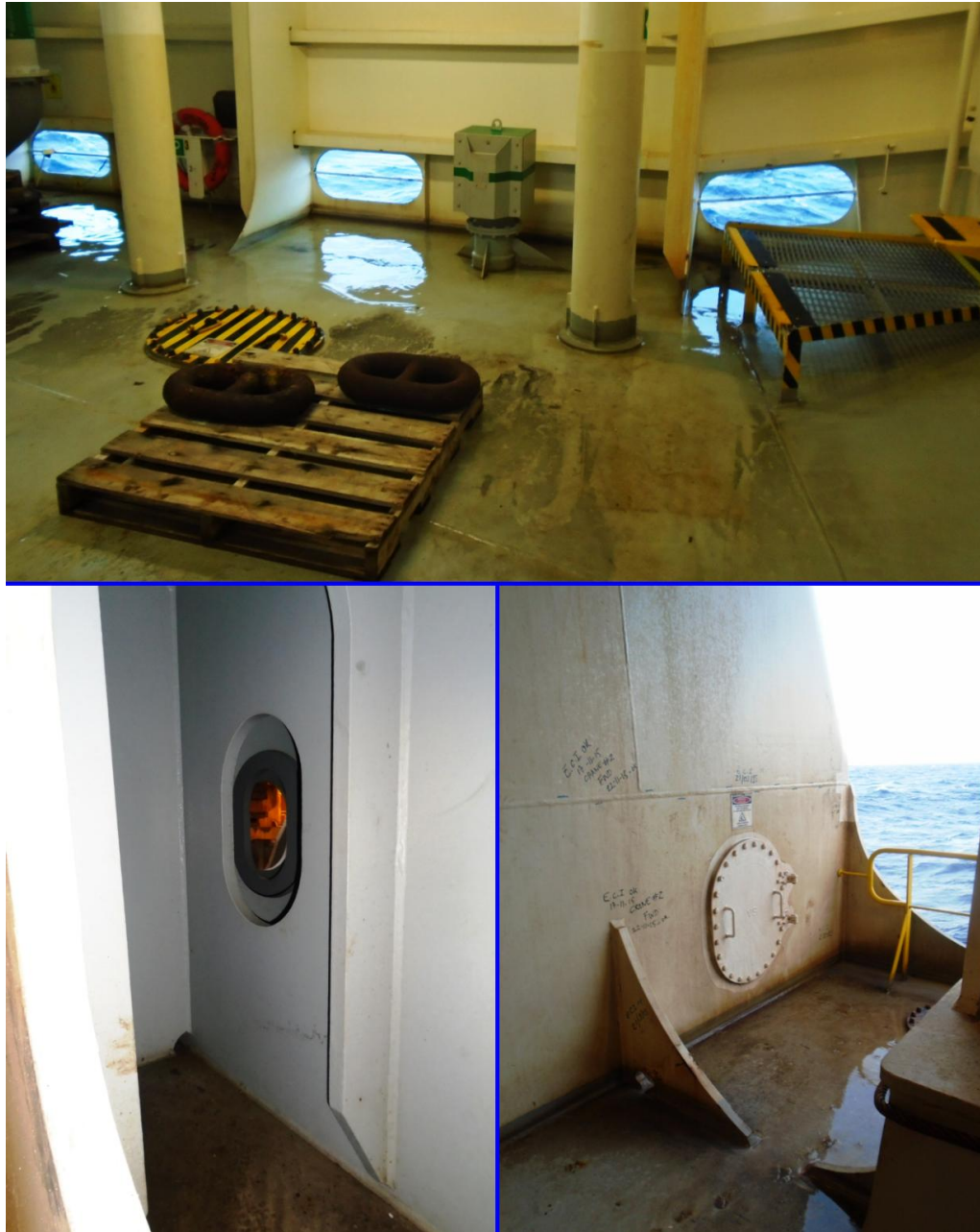
Figure 1. Oblong holes in offshore structures.
